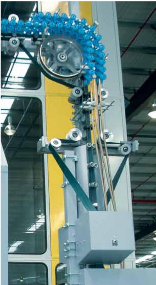
Infeed station and vertical conveying section
